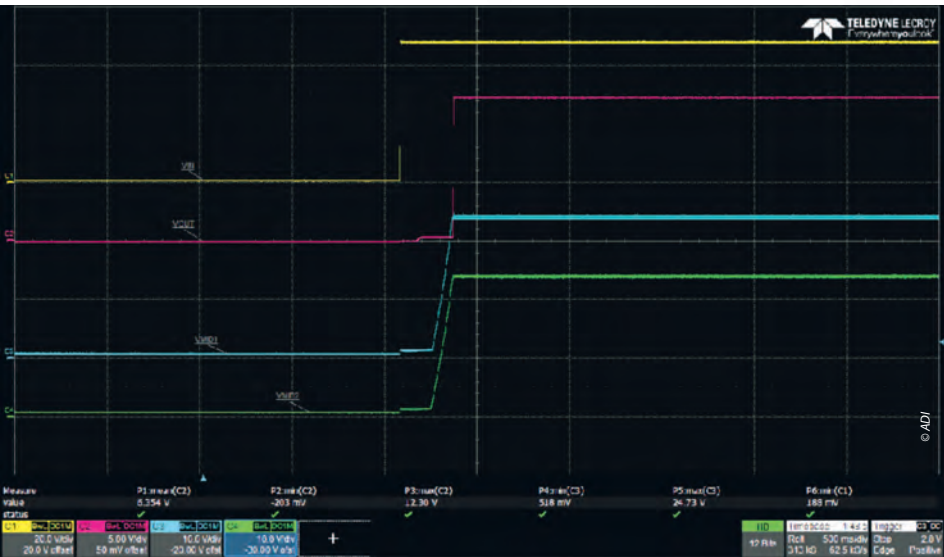
Figure 5 Hybrid converter startup at no load condition.
