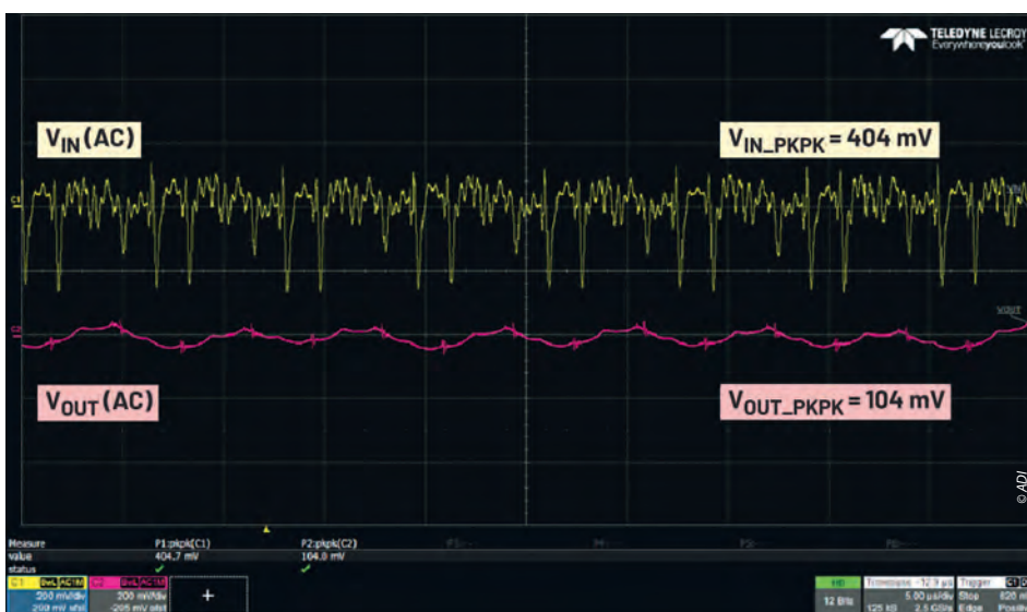
Figure 7 Input voltage ripple and output voltage ripple.
