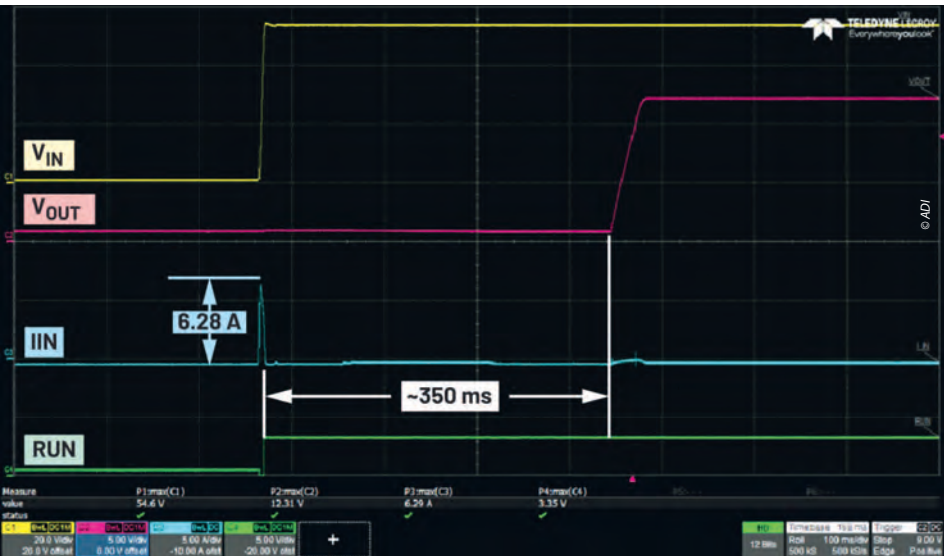
Figure 6 QBS startup at no load condition.
