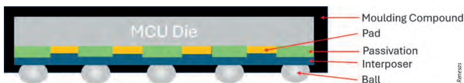
Figure 1 Simplified Internal structure of the WLCSP package.
