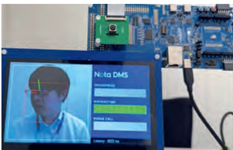
Figure 7 Driver Monitoring System on RA8P1 and Performance Comparison, NPU vs. CPU.
