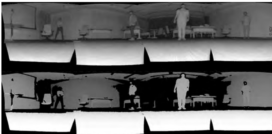
Figure 9 Stitched IR and depth image with 278° FoV.
