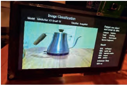
Figure 6 Image Classification on RA8P1 and Performance Comparison, NPU vs. CPU.
