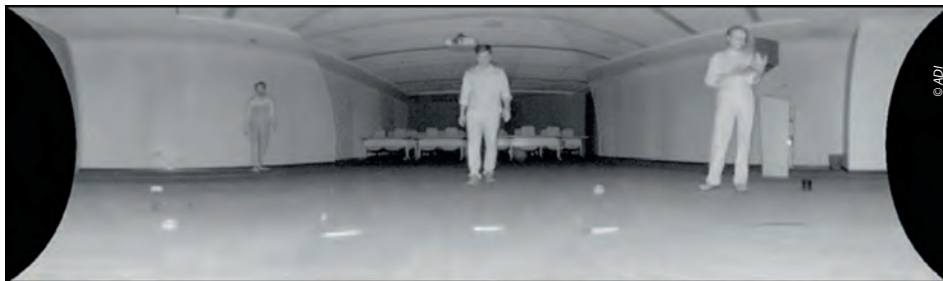
Figure 8 Stitched IR data giving a 210° FOV.
