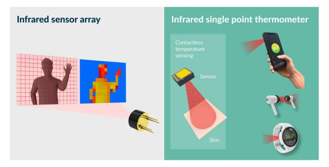
Melexis thermal imager ICs measure object temperatures from -40°C to 300°C with typical accuracy of ±1°C across its range. Its 32x24 pixel array can also be used for sophisticated AI-backed operations such as person and gesture recognition, providing a cost-effective and accurate way to improve robotic navigation and guidance.
