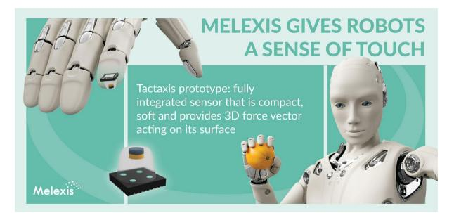
The sensor's construction enables it to measure normal forces up to 5 N and shear forces up to 2 N with impressive precision at the sensor level. A force resolution of 30 mN allows robots to detect weight changes as small as 3 grams, improving their ability to sense subtle force variations and dynamically adjust their grip and manipulation. This is particularly advantageous in applications such as stationary articulated arms, where
